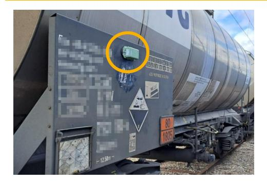
The proposal is to opportunistically use the Track Value solution and its internal sensors (accelerometer) for flat wheels detection.
